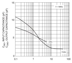
V<sub>CB</sub>, COLLECTOR-BASE VOLTAGE (V) Fig. 2, Input and Output Capacitance vs. Collector-Base Voltage
