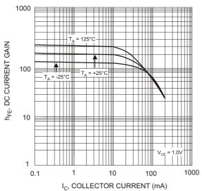
Fig. 3, Typical DC Current Gain vs Collector Current
